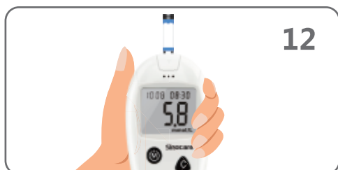
STEP 12: After a 10-second count down, the meter displays the test result.
