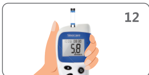
STEP 12: After a 9-second count down, the meter displays the test result.
